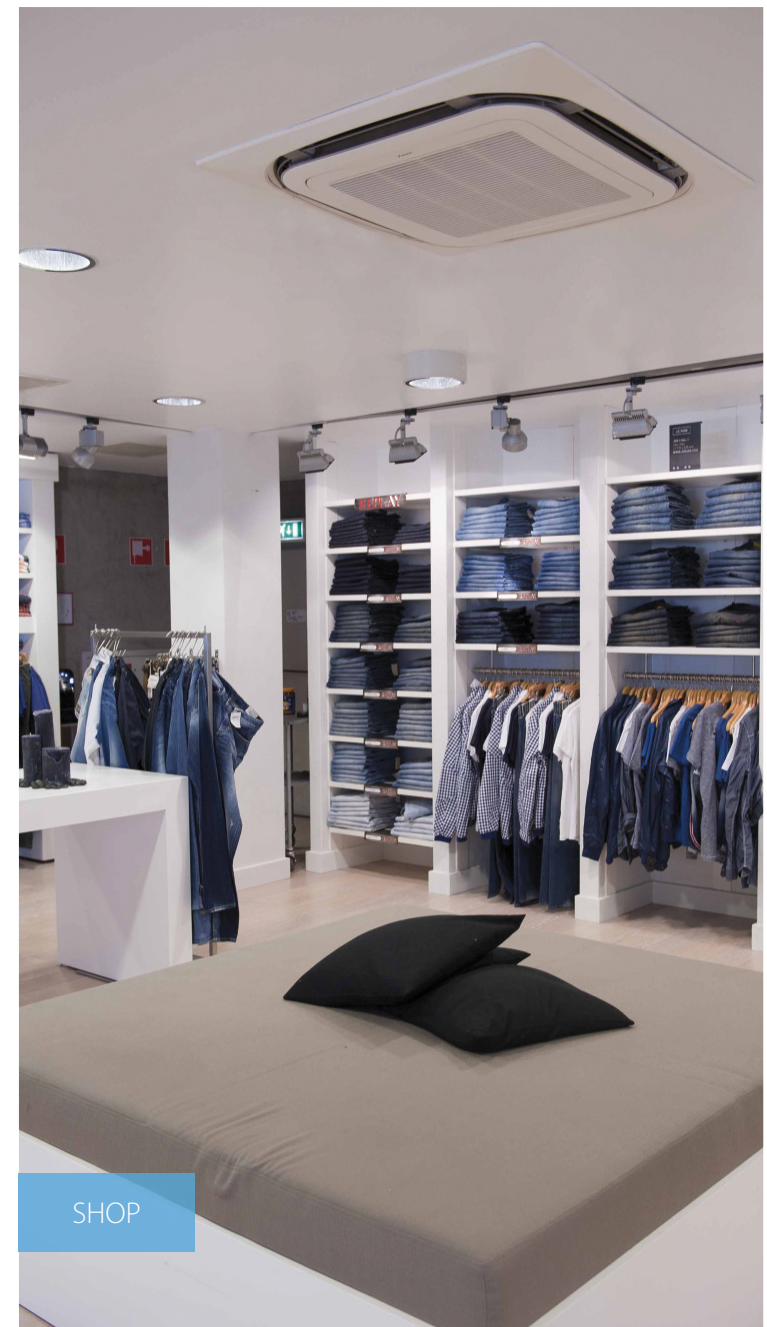
Round flow cassette FXFQ-A: 360° air discharge for optimum efficiency and comfort
