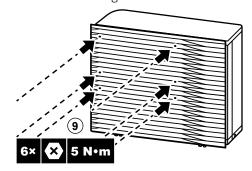
7.3.7 To remove the discharge grille, and put the grille in safety position
