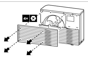
**2** Remove the lower part of the discharge grille.
