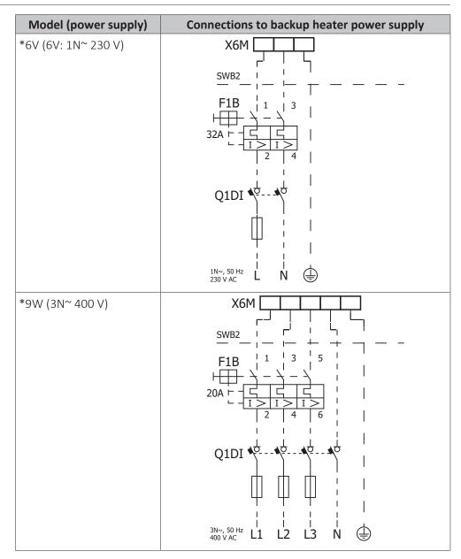
F1B Overcurrent fuse (field supply). Recommended fuse: tripping class C.
