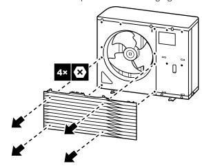
Rotate the lower part of the discharge grille.
