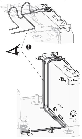
All cables which will be connected to the switch box of the  $\mathrm{ECH_2O}$  must be fixed by strain relief.
