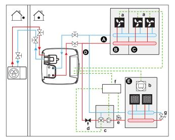
2 System with hydraulic separator for main zone:
