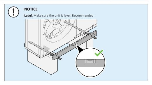
Use 4 sets of M12 anchor bolts, nuts and washers. Provide at least 150 mm of free space below the unit. Additionally, make sure the unit is positioned at least 100 mm above the maximum expected level of snow.
