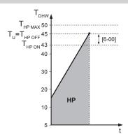
**HP** Heat pump. If heating up time by the heat pump takes too long, auxiliary heating by the backup heater can take place
