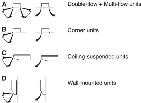
For the following conditions, a micro computer controls the air flow direction which may be different from the display.
