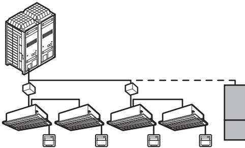
When the system is installed as shown in the figure above (one branch selector (BS) unit is connected to several indoor units), it is necessary to designate one of the remote controllers as the master remote controller.
