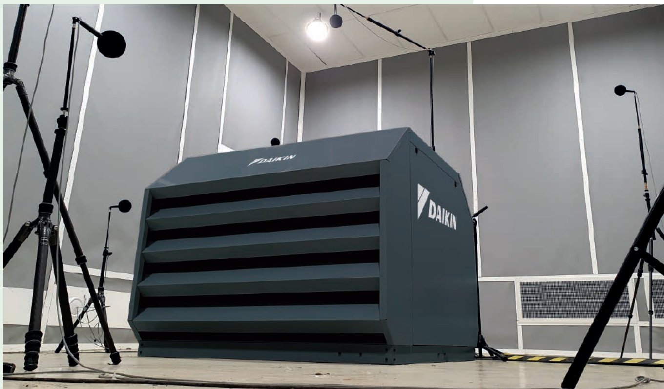
Sound power level measurement in acoustic chamber
